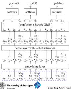
GRU-based cnet en- $S_i, U_i$ : coder outputs at the end of each system and user utterance
